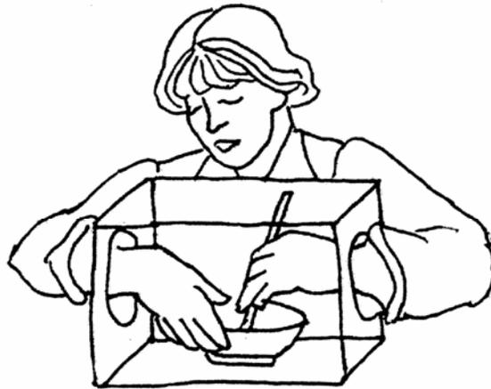
Figure 3: Glove Box for Mixing Powders
